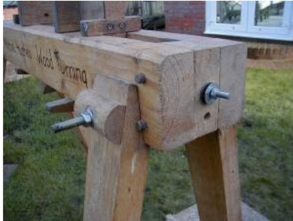
The best way to assemble this arrangement is shown in this picture. The bed is laid upside-down and the legs and bolts fed through the holes and tightened up before uprighting the lathe. Ignore the notches in the legs in the picture, these are from a previous experiment, however you should drilled a 12 mm hole near the basis of each leg so all the legs can be bolted together for transport, the picture of all the parts shows the legs bolted together.
