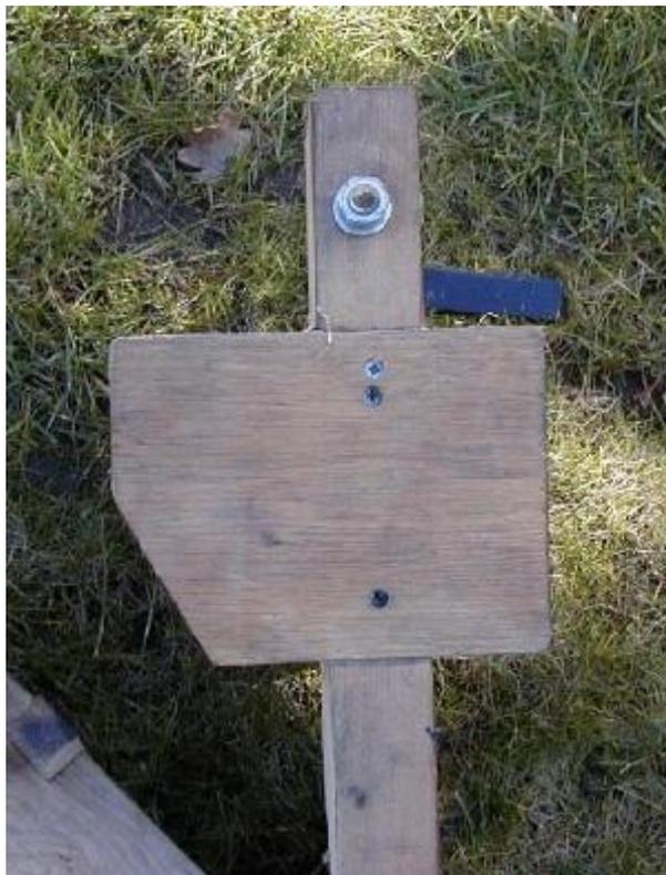
Note how the tool rest support extends further on one side to hold the tool rest. The poppets should mirror each other in this respect.
