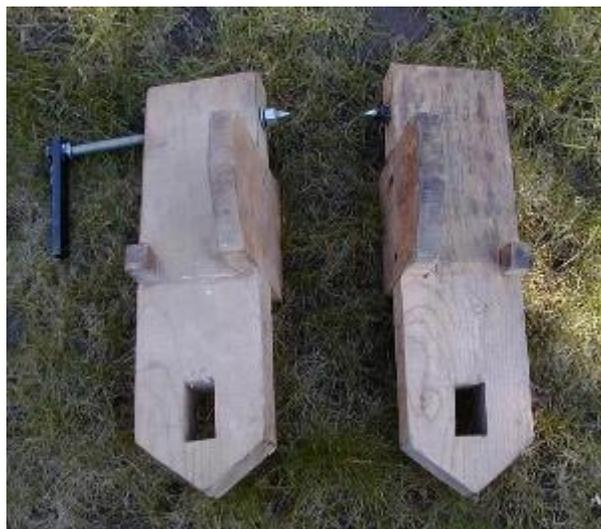
are held in place on the lathe bed by using hardwood wedges that you tap through holes in the poppets. The wedges are about 300 mm long and tapered at about 15 degrees. The holes in the poppets should overlap the underside of the bed so the wedges can be tightened against the lathe.
