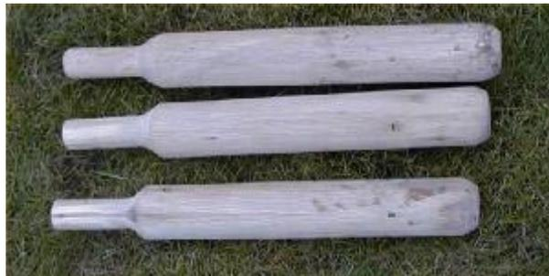
As the bed is softwood I doubled up on the thickness for the leg pins. Also notice the angle of the legs to increase stability.
