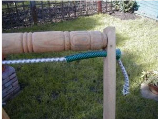
The top of these uprights are drilled 25 mm and a shoulder turned on the end of the spacer pole. No other fixing is required as the action of the bungee is to pull the uprights onto the spacer
