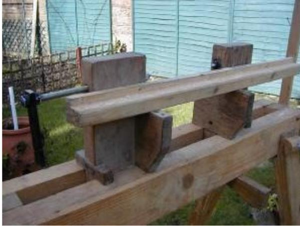
To make the crank at the end of the movable point, either bend the studding over, weld a handle on, or bolt a length of bar between two nuts.
