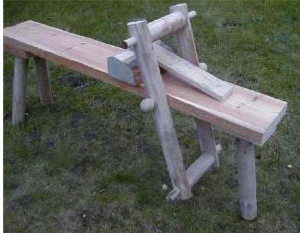
The shave horse can be disassembled in about one minute, however once the legs are removed the frame folds reasonably flat so I tend to leave it attached to the bed.
